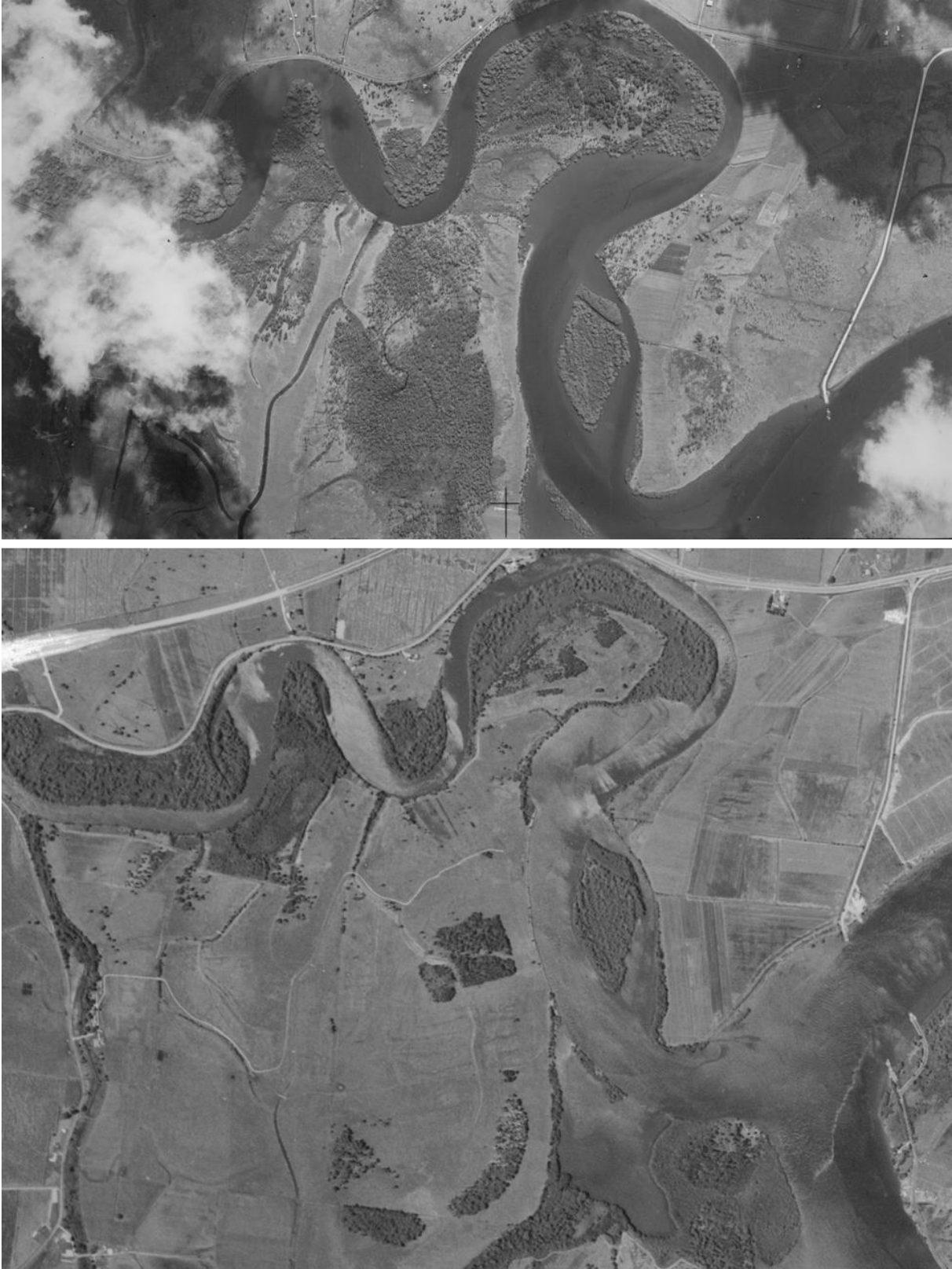
Figure 1.3: Historical aerial images of the Duck Creek site from 1942 and 1966, depicting the drainage works undertaken onsite.
